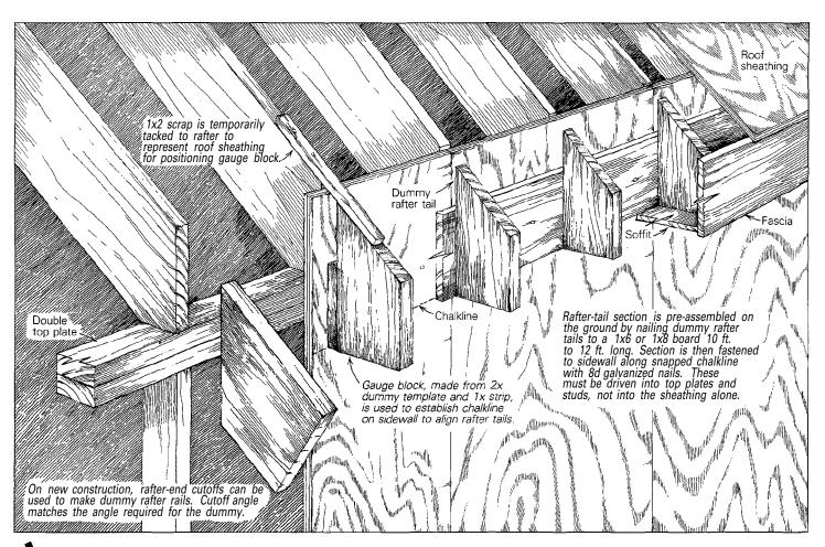
leaky roof or a backed-up gutter often leads to eaves and rafter tails that are badly deteriorated. On older houses, there's simply nothing solid to nail new fascia and soffit trim to. To deal with this problem, 1 cut the old rafter tails back flush with the siding, nail dummy 2x6 block rafter tails to a 1x board, and nail this in turn through the sheathing to the top plate, the cut-back rafter ends, or to both.
